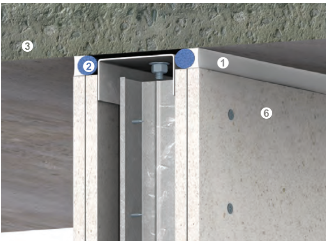
Typical head joints of lightweight partition (STC 45-50)
